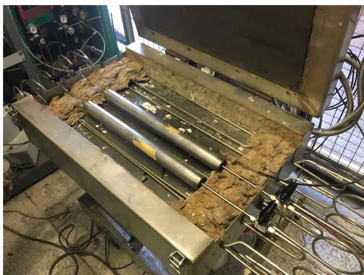
Figure 13.2: Two filters connected to a gas line and placed in the oven.
