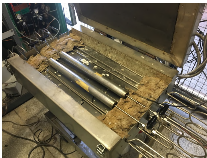
Figure 13.2: Two filters connected to a gas line and placed in the oven.
