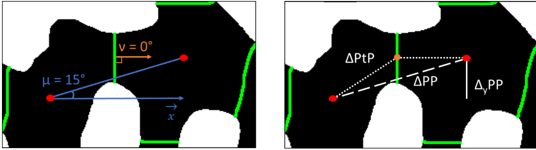
Figure 4-3: Visual description of some throat features. Pores are shown in black separated by throats in bright green. Pore centers of mass are shown as red circles. The throat orientation angle v is given by the angle between the normal to the throat (shown in orange) and the positive pressure gradient, in this case v is equal to 0. The orientation the neighboring pores centers of mass in relation to pressure gradient is given by the angle \mu . The distance from neighboring pores centers of mass is given by \Delta PP (shown in thickly dashed white). The total distance between the centers of mass passing by the throat center is given by \Delta PtP (shown in thinly dashed white).
