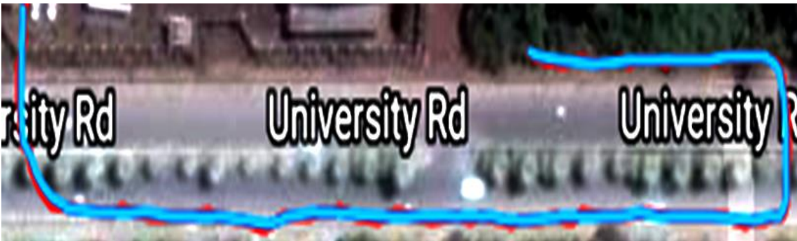
Figure 4.6: Smoothing of GPS reading by applying Kalman filter
