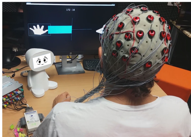
Figure 4.1: A participant training to use a BCI. He is learning how to perform different MI tasks (imagining a left-hand movement, performing mental calculation tasks and imagining an object rotating) to control the system. Along the training, PEANUT (on the left) provides users with social presence and emotional support, using interventions composed of facial expressions and pronounced sentences adapted to their performance and progression.
