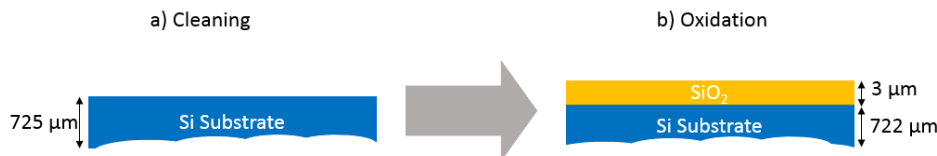
Figure 33- Schematic of 3 \mu\text{m} oxidation.
