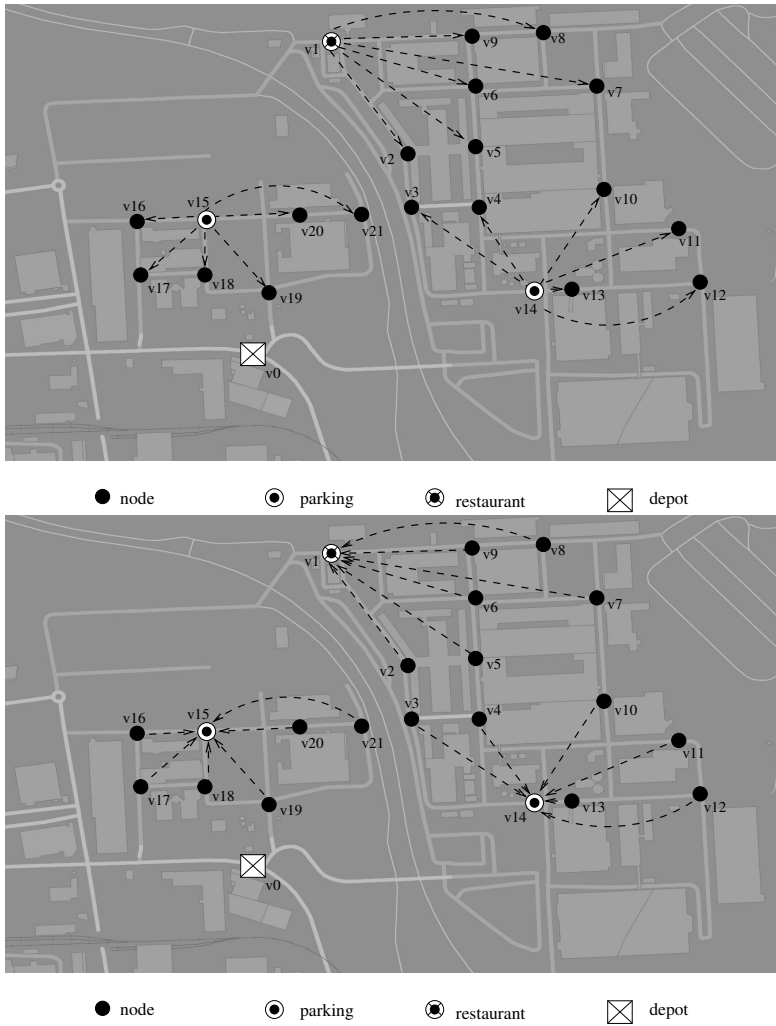
Figure 3.2: This figure illustrates an example of the morning respectively evening pattern of requests on the network G of the industrial site “Ladoux” of Michelin at Clermont-Ferrand. Each station is highlighted by a dot on the map; the different parkings are illustrated by a black dot within a white dot. The depot of the network is illustrated by a cross within a square. The transportation requests of the customers are indicated by arcs from the origin to the destination.
