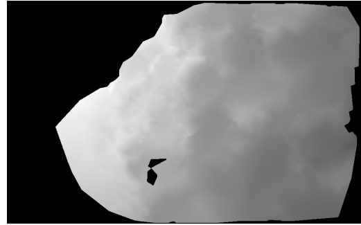
(B) 2D densified depth map from the Delaunay-based interpolation.
