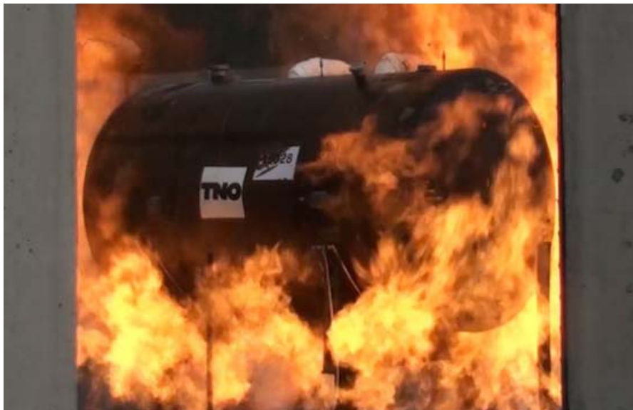
Figure 1.5: Double walled tank containing cryogenic liquid engulfed in fire during the experiment, from [4]
