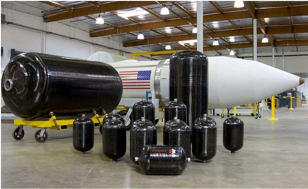
(a) Composite tanks, credit: ABS [39]
