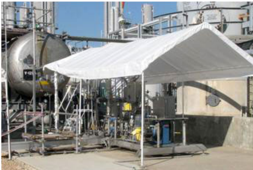
(b) Compact sulfur reduction unit, from [26]
