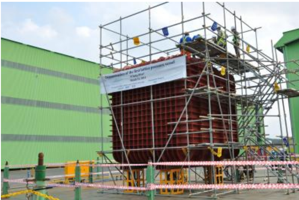
(b) Prototype of a box-shaped pressure tank, credit: KAIST [40]
