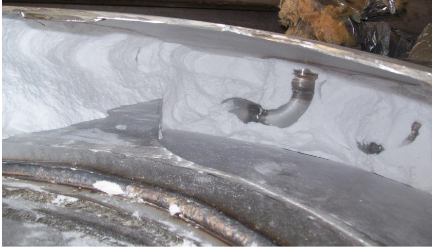
Figure 1.6: Vacuum space with perlite filling, from [5]
