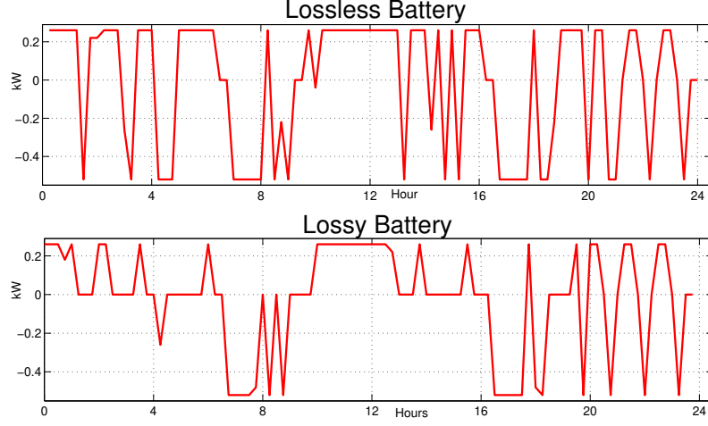
Figure 5.2: Comparison of ramp rates for same price signal without and with efficiency losses
