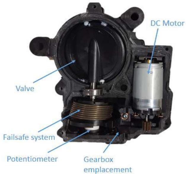
Figure 3-6. Siemens VDO model
