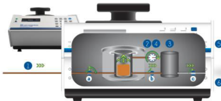
Figure 25. Measuring density with the Micromeritics pycnometer. [194]
