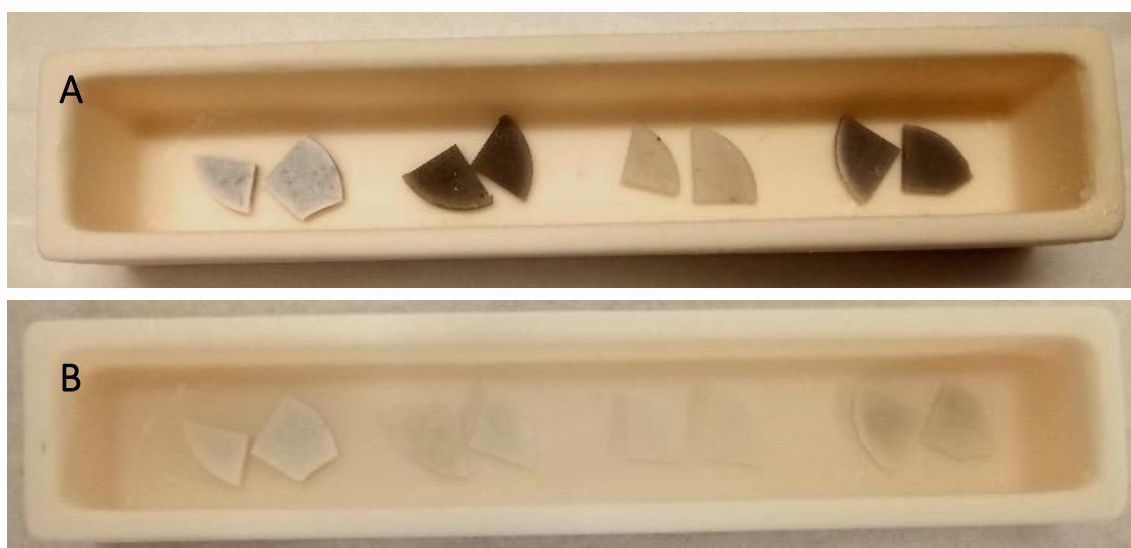
Figure 65. A: 2c, 5c, 9c and 12c samples after 30-minute 1300°C annealing in air; B: Samples after additional 4-hour annealing under oxygen flow at 1350°C.
