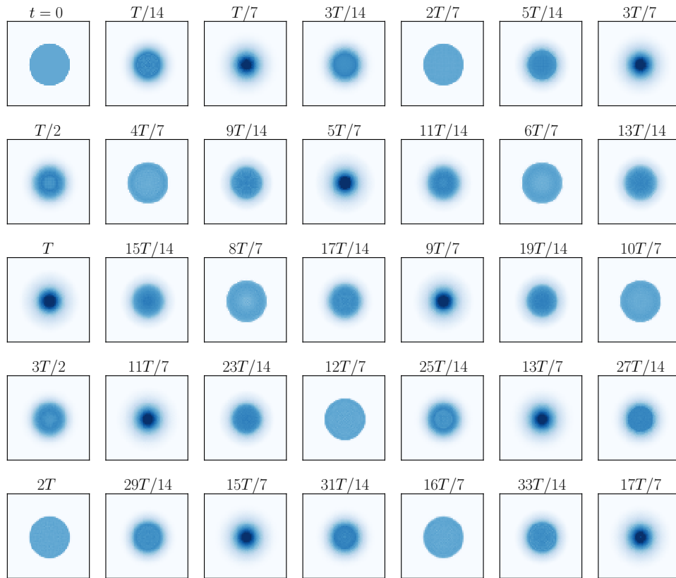
Figure 9.9: Numerical simulation with an initially uniform disk-shaped cloud, for the parameters N_s = 512 and \alpha = 4 . The initial wave function is the ground state of a disk-shaped box-potential. The images show the density distribution of this wave function during an evolution according to the full Gross-Pitaevskii equation. The same density distribution seems to appear every 2T/7 .
