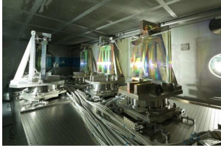
Fig. 19. Picture of three out of four full size multilayers diffraction gratings facing their paired gratings implemented in the final (vacuum) compression stage
