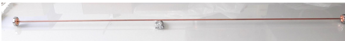
Figure 7.3. 5mm diameter, 1.2 meters length, NEG coated chamber.
