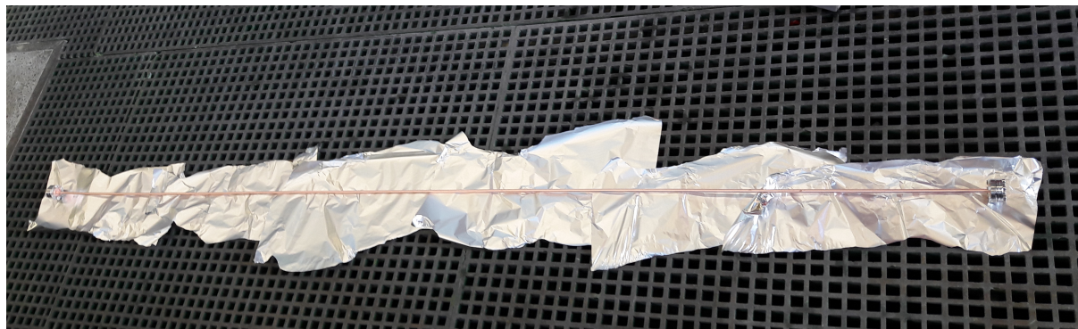
Figure 7.5. 4mm diameter, 2 meters length, NEG coated chamber.
