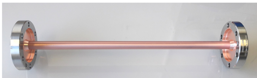
Figure 2.5. Coated mandrel and stainless steel flanges mechanically assembled prior to electroforming.
