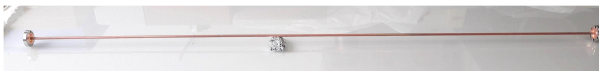
Figure 7.3. 5mm diameter, 1.2 meters length, NEG coated chamber.
