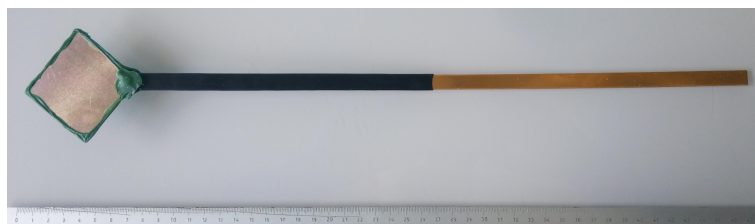
Figure 5.7. Platelets after copper PVD coating, before electroforming.
