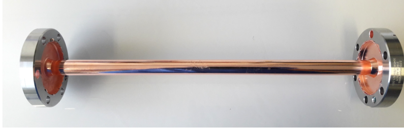
Figure 2.7. Electroformed chamber with the stainless steel flanges assembled using DC plating in the bath that contains a brightener.
