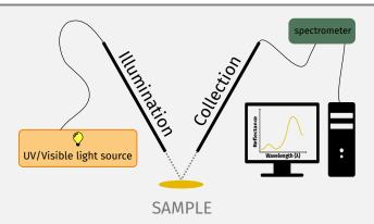
Figure 1.4: Drawing of a set-up to measure spectral reflectance from a sample: the light is brought from a lamp to the sample via an optical fibre (illumination fibre). The light reflected by the sample is then collected by a second optical fibre (collection fibre) which brings it to the spectrophotometer.
