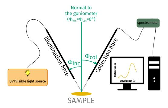
**Figure 1:** Schematic representation of a goniometer with the illumination and collection fibres and their angle with the normal to the sample  $\Phi_{inc}$  and  $\Phi_{col}$ . The sign of  $\Phi_{inc}$  and  $\Phi_{col}$  is figured by an arrow pointing towards the positive rotation direction.
