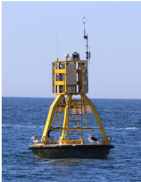
*Figure 1-1: A met-ocean buoy installed at the SEM-REV site.*
