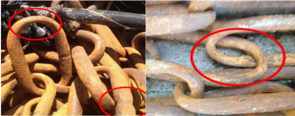
*Figure 2-31: Corroded chain mooring lines of a met-ocean buoy at the SEM-REV sea test site (Berhault, 2017).*
