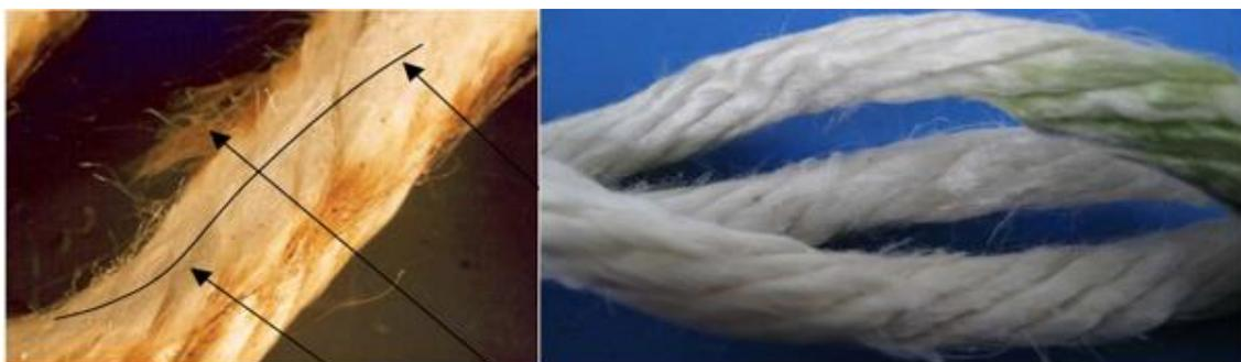
Figure 2-12: Inter-strand damage in a polyester rope (left) after a 48-million-cycle fatigue test (Banfield et al., 2018) and a nylon subrope (right) after a ten-million-cycles fatigue tests (Banfield et al., 2017).
