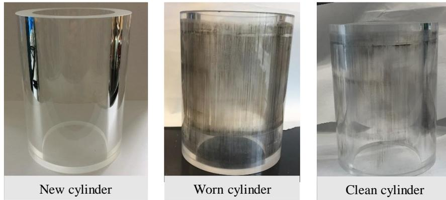
Figure 5-10: Wear of the transparent cylinder after the acquisition of three data sets corresponding to 600 engine cycles. Note the intensity of black traces on the cylinder walls.
