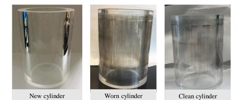
Figure 5-10: Wear of the transparent cylinder after the acquisition of three data sets corresponding to 600 engine cycles. Note the intensity of black traces on the cylinder walls.
