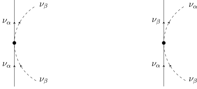
Figure 2.5: Illustration of the interaction terms in Eq. (2.92) corresponding to the mean-field approximation for the neutrino self-interaction terms. Background neutrinos are illustrated as dashed arcs, while the test neutrino is a solid straight line. The left panel corresponds to the diagonal contributions, and doesn't involve a flavor change. The right panel corresponds to the off-diagonal contributions and makes the test neutrino change its flavor. Antineutrinos also contribute to these terms.
