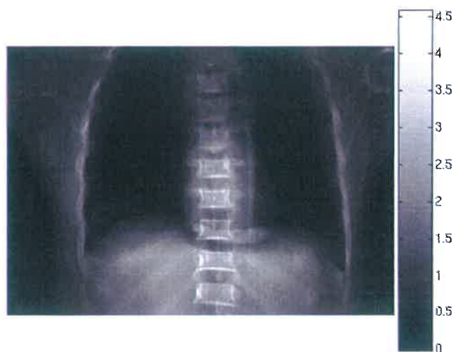
Figure 3: Ratio between scatter spatial distribution and primary radiation image on the detector area for an AP radiographic acquisition of the anthropomorphic thorax phantom.
