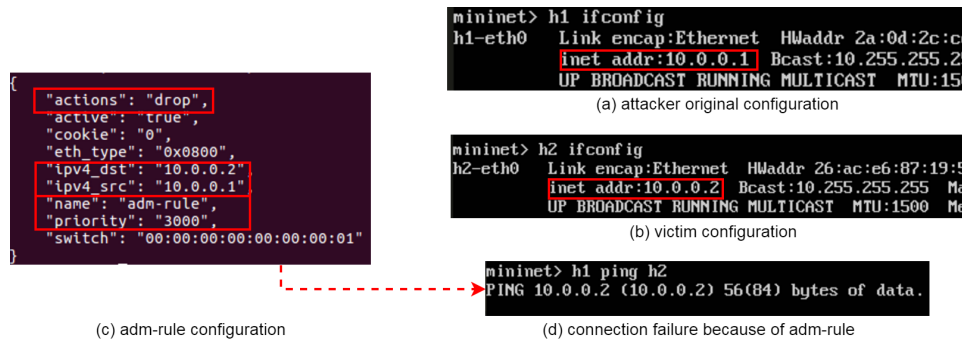
Fig. 4.20 Initial configuration and connection before priority-bypassing attack
