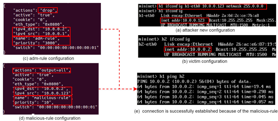
Fig. 4.21 Priority-bypassing attack success on the controller Floodlight
