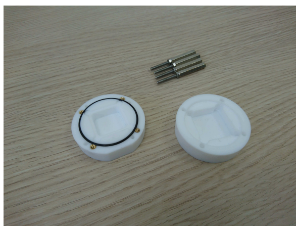
Figure II.2.6 – Solid/liquid cell used for AFM experiments on double lipid bilayers prepared by LB and LS depositions.
