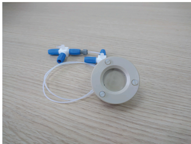
Figure II.2.12 – Solid/liquid cell for fluorescence microscopy experiments.
