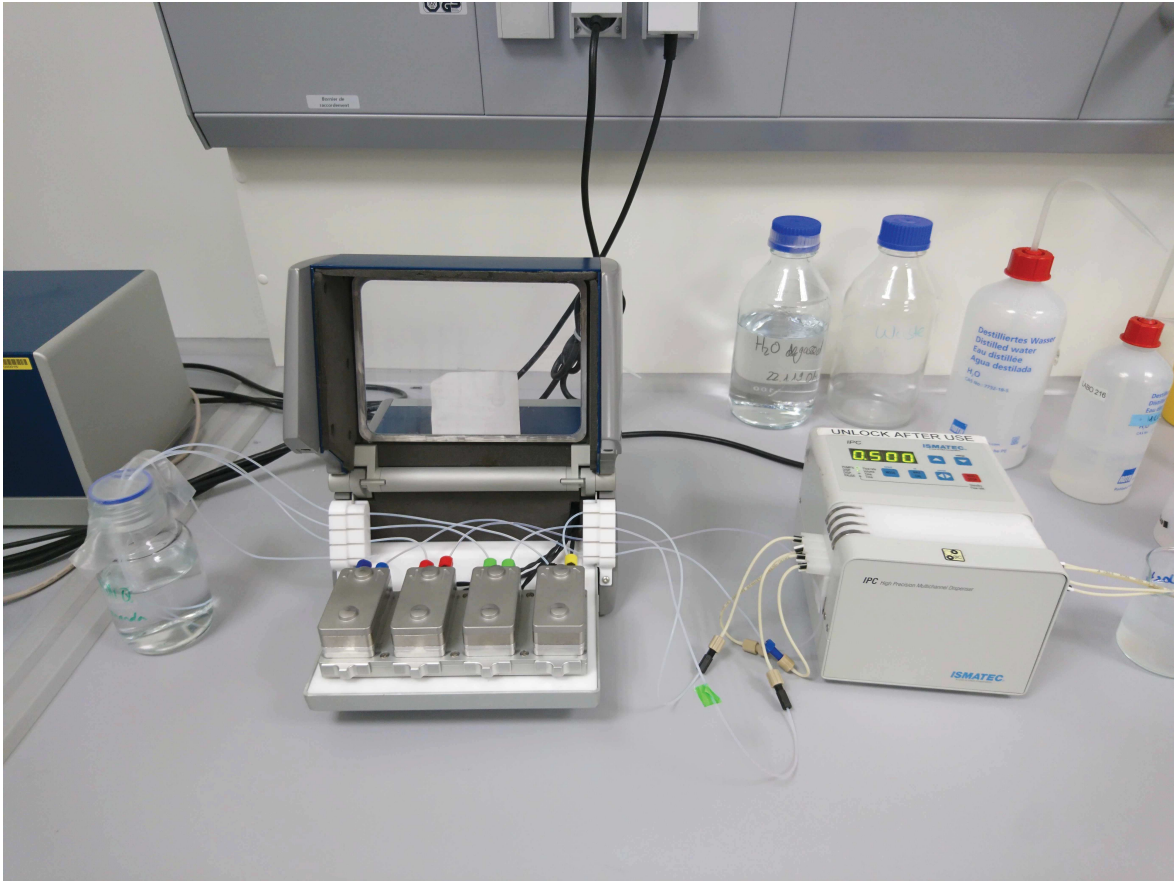
Figure II.2.3 – QCM-D Q-Sense series E4 instrument used in this thesis.
