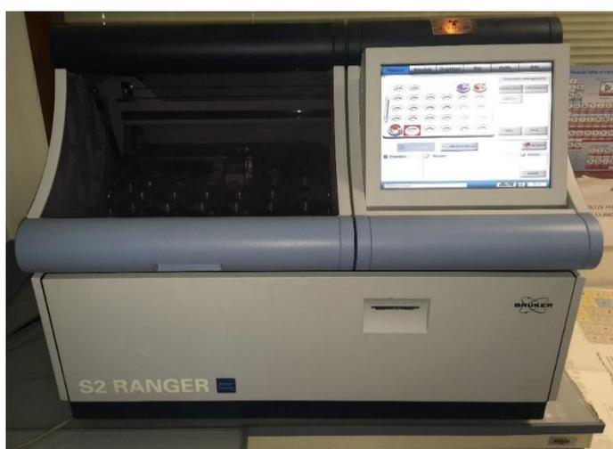
*Figure 25: Appareil de Fluorescence X Bruker S2 Ranger*
