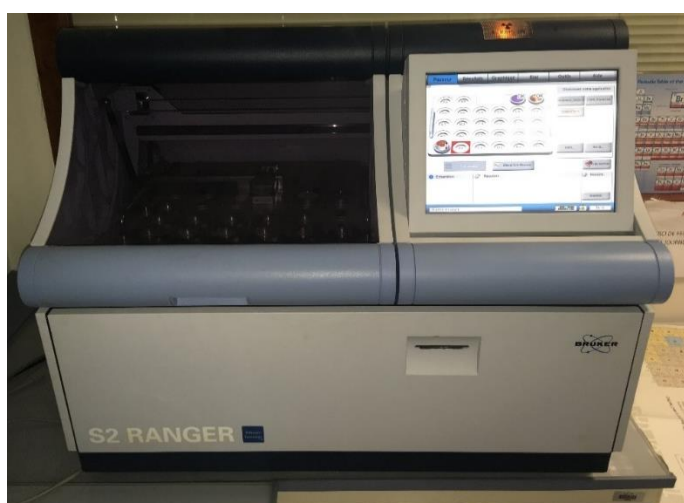
Figure 25: Appareil de Fluorescence X Bruker S2 Ranger
