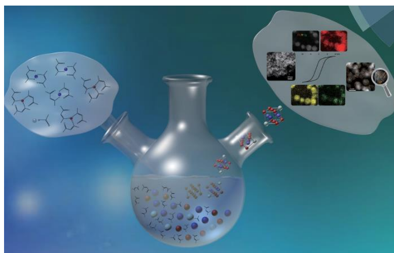
Fig. 2.3 Illustration of one-pot method for synthesis of metal nanoparticles. The reactants containing metal precursors, stabilized agents, reductants and solvent are all put into a vessel. After successive multistep chemical reactions of decompositions or reductions, metal nanocrystals are obtained. 118
