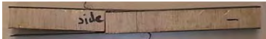
FIGURE 50 – Rupture de composite à âme balsa [Abo00].
