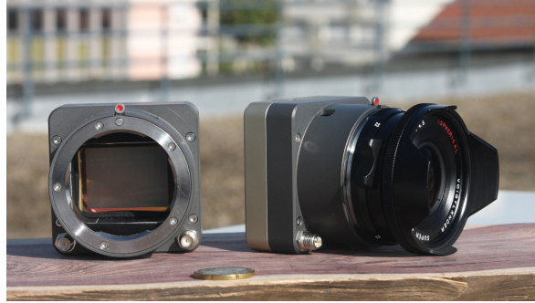
Figure. 3.4 – CamLight, the light metric camera for UAV applications developed at IGN.
