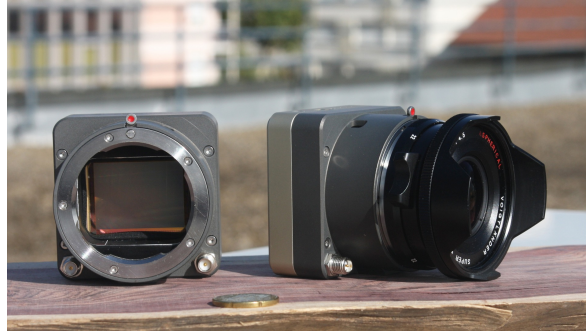
Figure. 6.1 – CamLight, the light metric camera for UAV applications developed at IGN.
