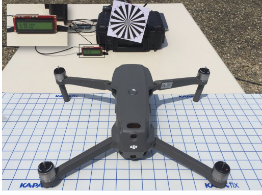
(a) The readout time calibration system
