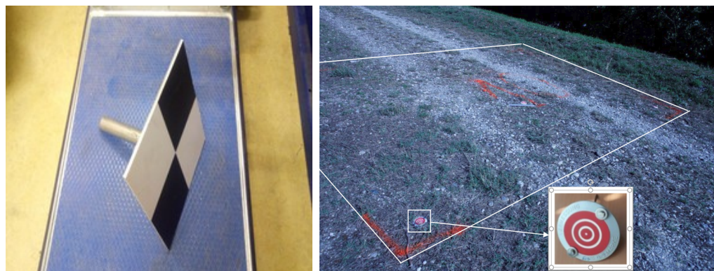
(a) Target serving as ground points
