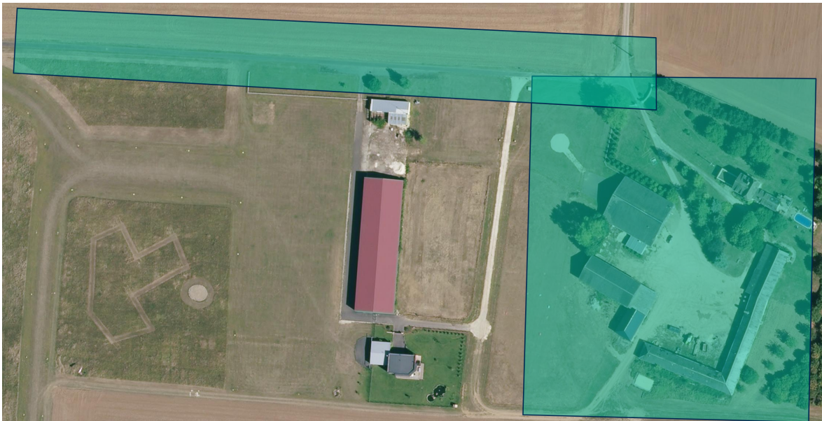
Figure. 7.12 – Illustration of the two surveyed zones in block and corridor configurations.
