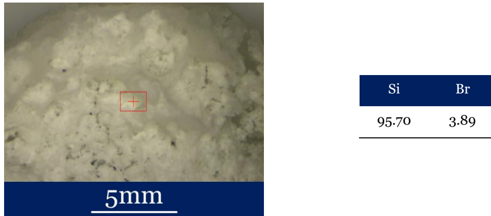
Figure III. 24: \mu -XRF analysis of the cured Si-loaded PU resin
