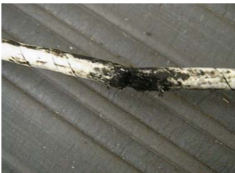
(a) Cut wire (Open circuit).
