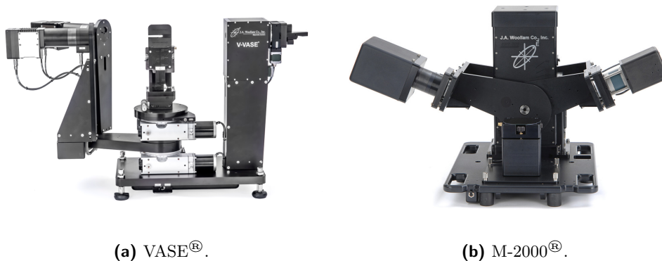
Figure 3.3: Ellipsometers adopted for optical characterisation. a) The VASE, with a vertical sample mount. b) The M-2000, featuring a horizontal sample mount. (© J.A. Woollam Co.)
