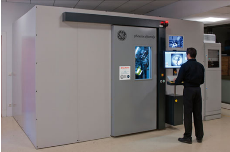
FIGURE 5.2: External view of the “v|tome|x L 240-180” industrial micro CT scanner, MNHN, Paris. Image taken from Sanz et al. (Sanz et al., 2013).
