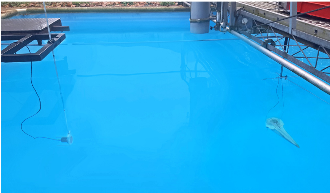
FIGURE B.6: Photograph of the experimental setup. The skull was placed 2 meters away from the loudspeaker and rotated around the vertical axis by the electronic rotation device.
