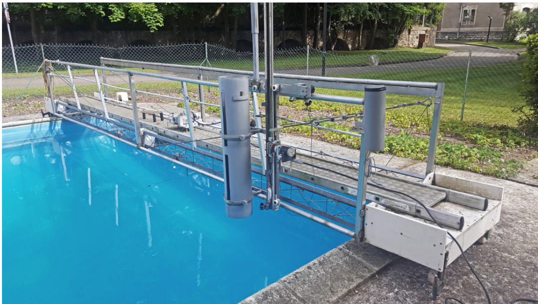
FIGURE B.5: Photograph of the rotation system. An electronic (house-made) rotation device was mounted on a large metal plank. The plank could be moved over the water and positioned at a desired distance away from the transducer.
