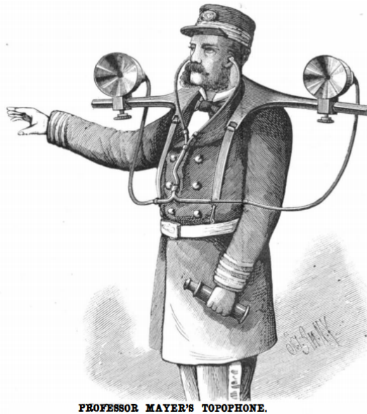
FIGURE 2.1: Professor Andrew Mayer and his invention - the topophone. This drawing appeared in the Scientific American in 1880 (Anonymous, 1880). The device was supposed to help the user in determining “[...] quickly and surely the exact direction and position of any source of sound” while navigating through fog (Mayer, 1880).
