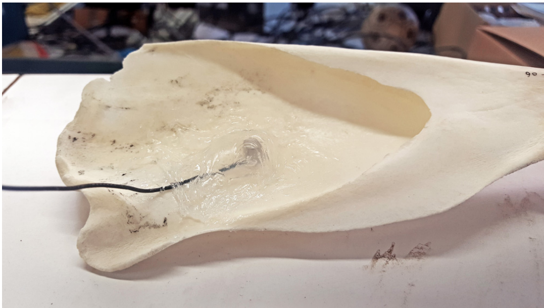
FIGURE B.3: Photograph of the accelerometer glued to the mandible. Each accelerometer was glued to the mandible with super glue and coated with flexible adhesive to keep water from touching the equipment.
