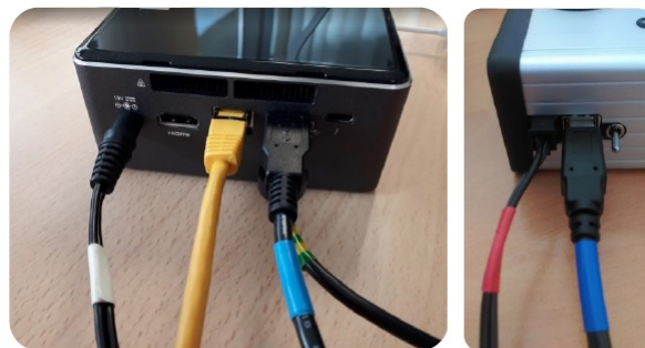
Figure 5.8 – Color marked wire connection to the computer unit (left) and to the device (right).
