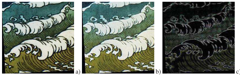
Fig. 6 Imprecise rotation by 3^\circ of the same detail of Figure 1. The interval-valued image is represented by its lower bound (a) and its upper bound (b). (c) is an enhanced view of the difference between the upper and the lower image, i.e. the imprecision of the interval-valued images.
