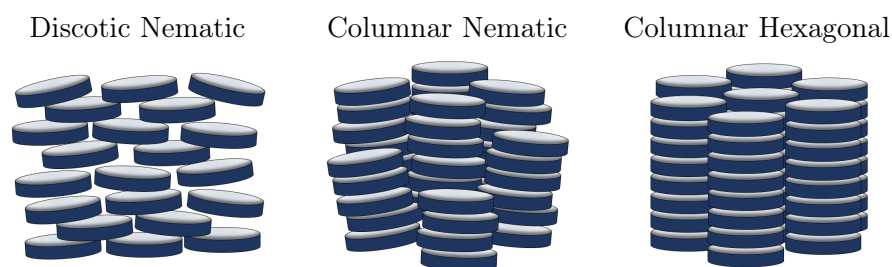
Figure 1.13 – Schematic representation of most common discotic mesophases: discotic nematic N_D , columnar nematic N_{Col} and columnar hexagonal Col_H
