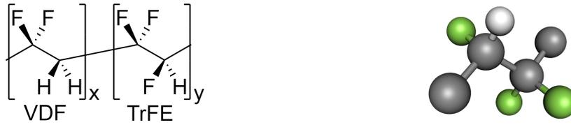
**Figure 2.12:** Chemical formula of the P(VDF-TrFE) copolymer and a 3D representation of the TrFE unit (grey: carbon, green: fluorine and white: hydrogen).
