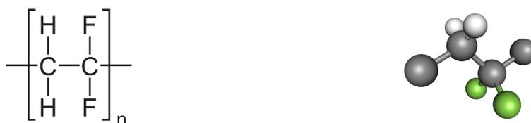
**Figure 2.9:** Chemical formula of the PVDF and a 3D representation of the VDF unit (grey: carbon, green: fluorine and white: hydrogen).
