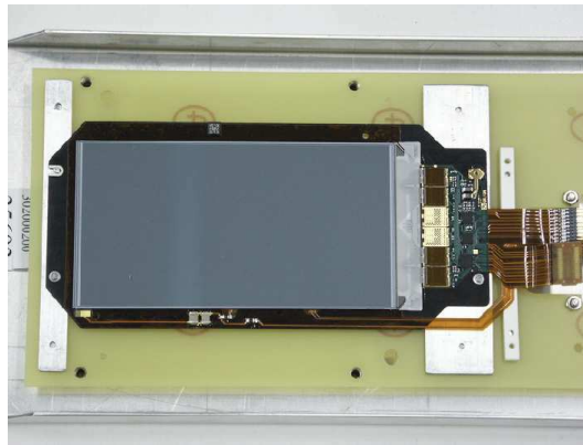
Figure 2.9: Single-sided TIB module. The 512 strips are read-out by 4 APV chips on the right-hand side. Taken from Ref. [158].
