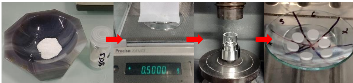
Figure 10. Procedure to prepare radio-opaque BG45S5 pellets following the norm ISO 13116:2014
