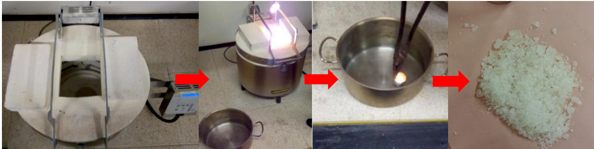
Figure 3. Melt and fast quenching procedure to fabricate BG45S5 using the Nebertherm Eco top-loader kiln
