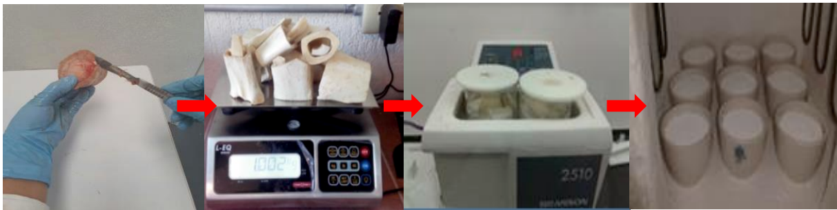
Figure 1. Procedure to obtain BHAp from bovine bones
