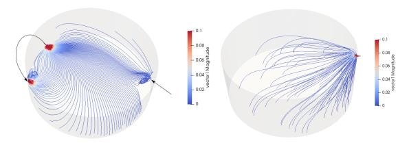
Figure 4.2: Streamlines of fluid flow, for standard operating conditions  $Q_r = 150 \text{ L/h}$  and  $Q_{mix} = 1000 \text{ L/h}$ . Bottom section (left) and top section (right).
