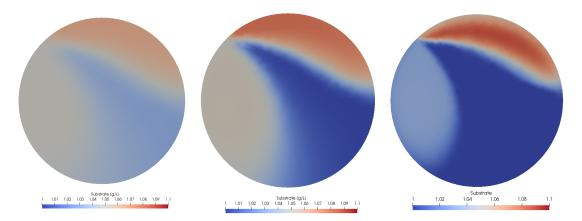
Figure 4.3: Bottom-Middle interface at 8h after a 10 % change of inflow concentration with mixing flow rate  $Q_{mix} = 1000 \text{ L/h}$  and different diffusion parameters. Left  $D = 10^{-6}$ , Center  $D = 10^{-7}$ , Right  $D = 10^{-8}$ .
