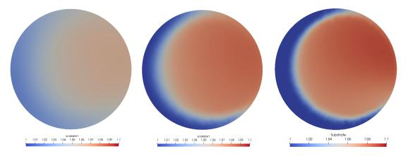
Figure 4.4: Bottom-Middle interface at 8h after a 10 % change of inflow concentration with mixing flow rate  $Q_{mix} = 0$  L/h and different diffusion parameters. Left  $D = 10^{-6}$ , Center  $D = 10^{-7}$ , Right  $D = 10^{-8}$ .
