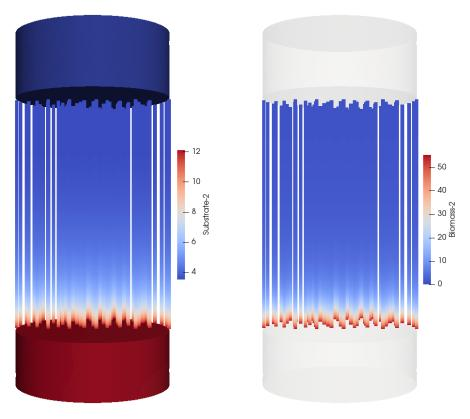
Figure 4.11: Distribution of  $S_2$  and  $B_2$  at steady state with  $Q_r = 50$  L/h.
