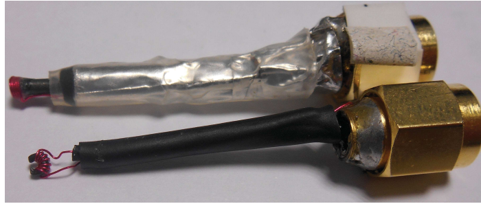
Figure 2.6: Examples of EMFI probes I used during my work
