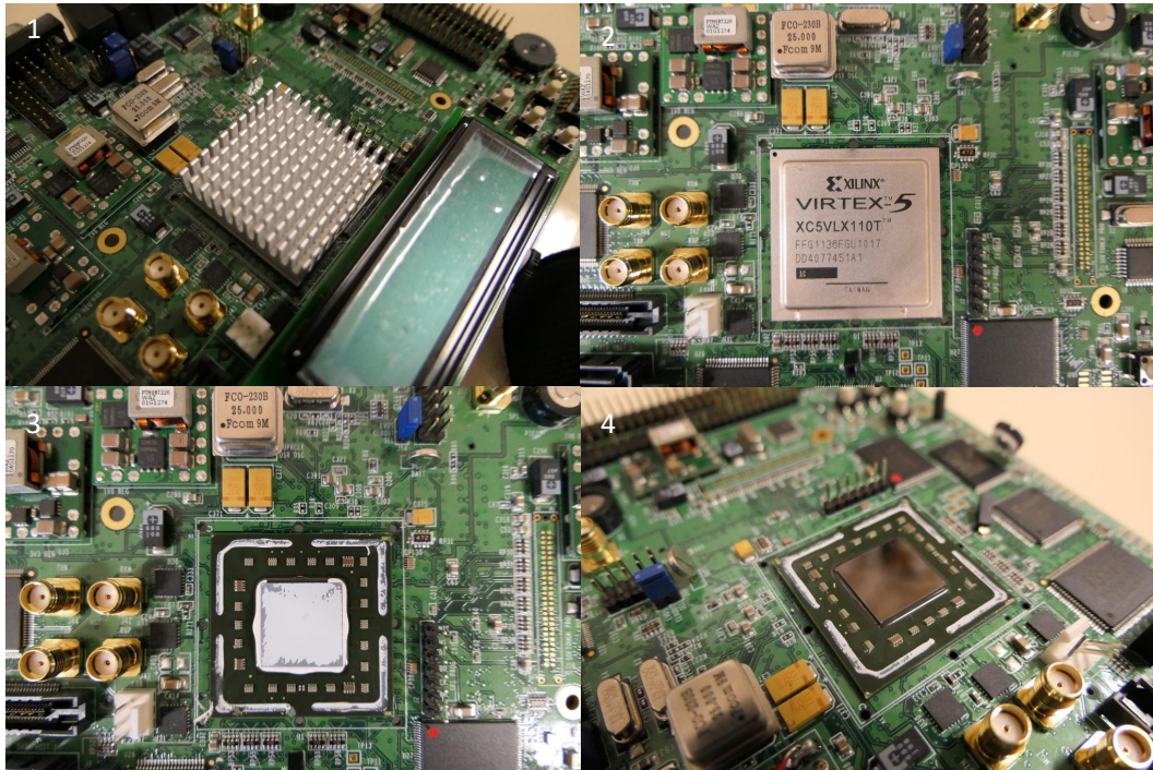
FIGURE 3.15: Decapsulation process of a flip-chip FPGA: 1. heat sink removal 2. uncapping the metal lid package 3. Cleaning the thermal paste of the silicon substrate 4. Final cleaned silicon die.
