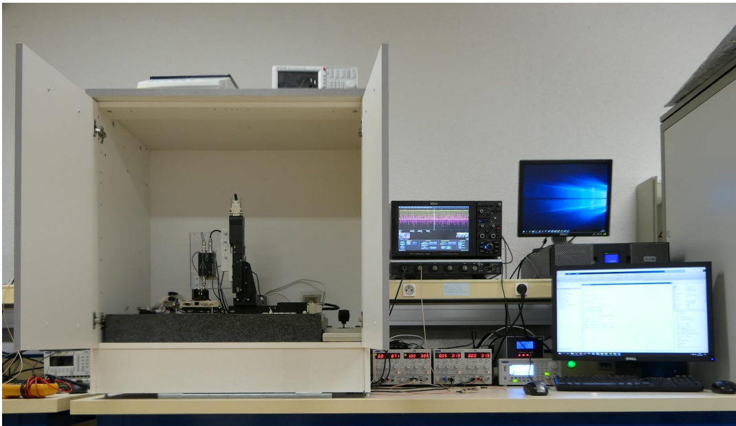
FIGURE 3.4: IR acquisition platform in its isolation container.
