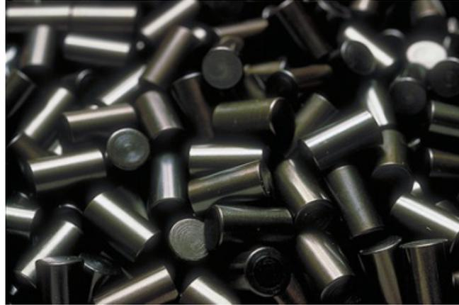
FIGURE 1.3: Fuel pellets used in the fuel rod. *Source: [4]*
