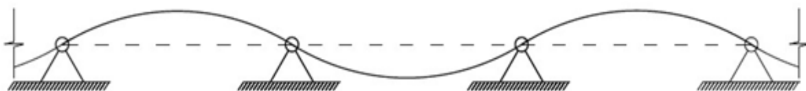
Figure 1.8 – Mode de vibration Pinned-Pinned d'un rail [2]
