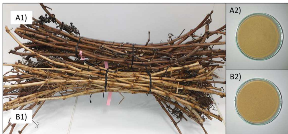
Figure 74. Pictures of 2018 vine shoots: Chardonnay (A1) and Grenache (B1), and fillers after impact milling: Chardonnay (A2) and Grenache (B2).
