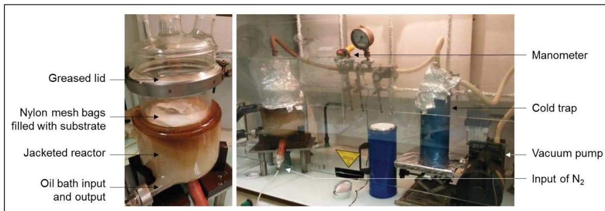
Figure 34. Experimental set-up of the gas-phase esterification
