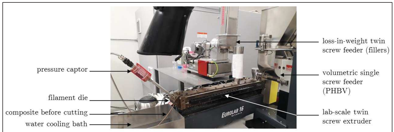
Figure 35. Melt extrusion set-up (here with a filament die)
